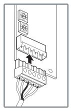
(5) When wiring the FR-E700 series, if a hook of the front cover of the plug-in option impedes wiring, cut off the hook and perform wiring.
