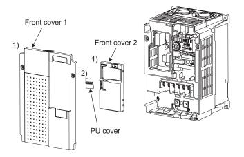
Because the voltage is stated on the PU cover, replace a PU cover of a plug-in option front cover with the removed PU cover from the inverter.
