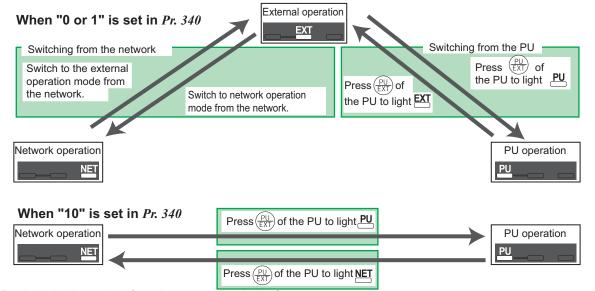
For the switching method from the external terminal, refer to *the inverter manual*. Refer to *page 72* for a switching method from the network.
